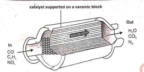
Catalyst systems of this type cost several hundred pounds, mainly because of the high cost of the precious metal they contain. The catalyst is poisoned by lead, so unleaded fuel must always be used.
